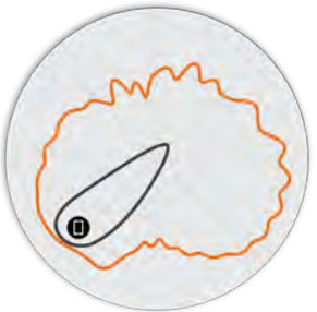
Figure 5. R350 5GHz Elevation Antenna Patterns
